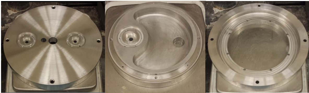
Figure 4.3. Fabricated components: 8in diameter top cap (lt), 5-3/4in diameter pump pickup (ctr), and 8in diameter bottom cap with recesses for housing and pickup plate (rt).
