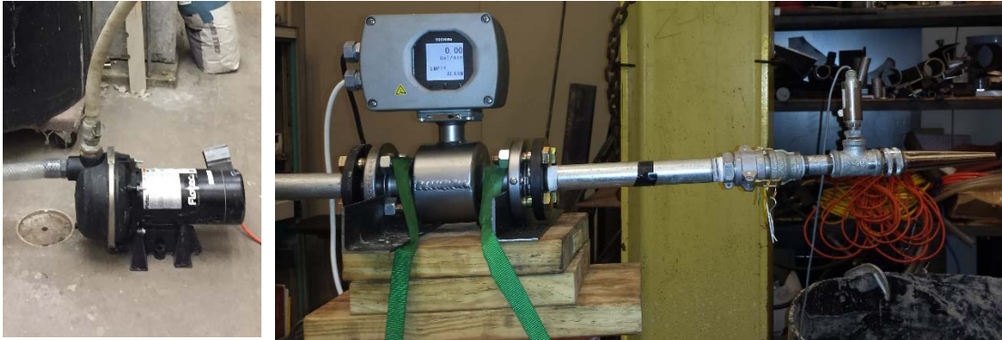
Figure 3.39. Pump (left), flow meter, pressure transducer and nozzle (right)
