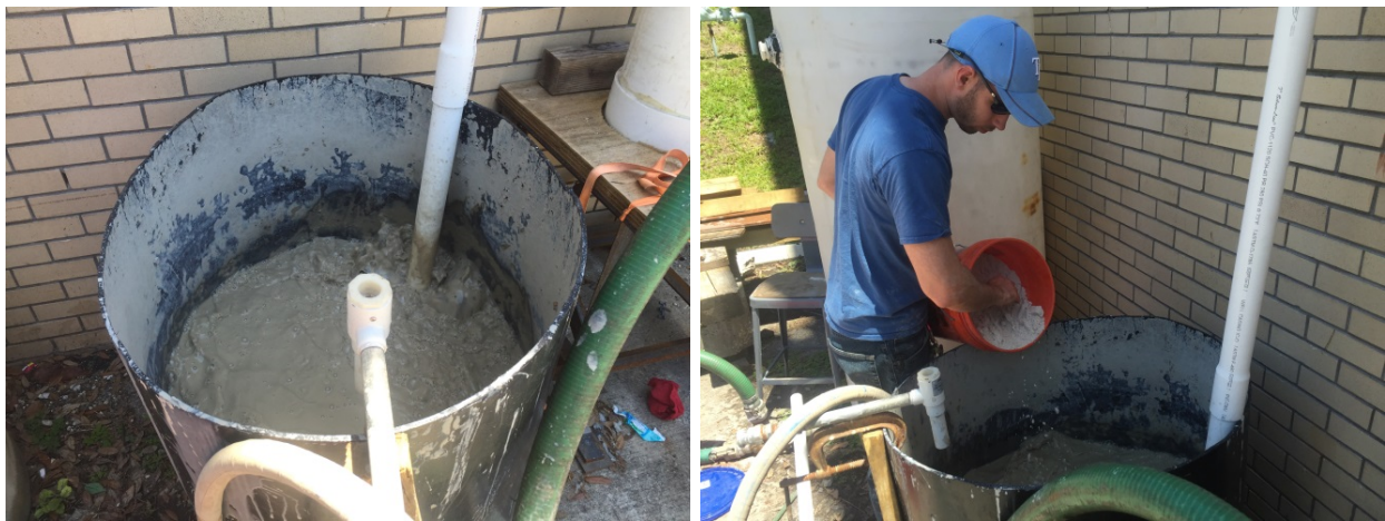
Figure 5.10. Increasing sand content by adding sand during slurry recirculation cycle.
