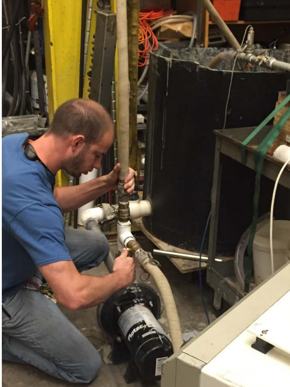
Figure 3.43. Adjusting slurry flow control valve
