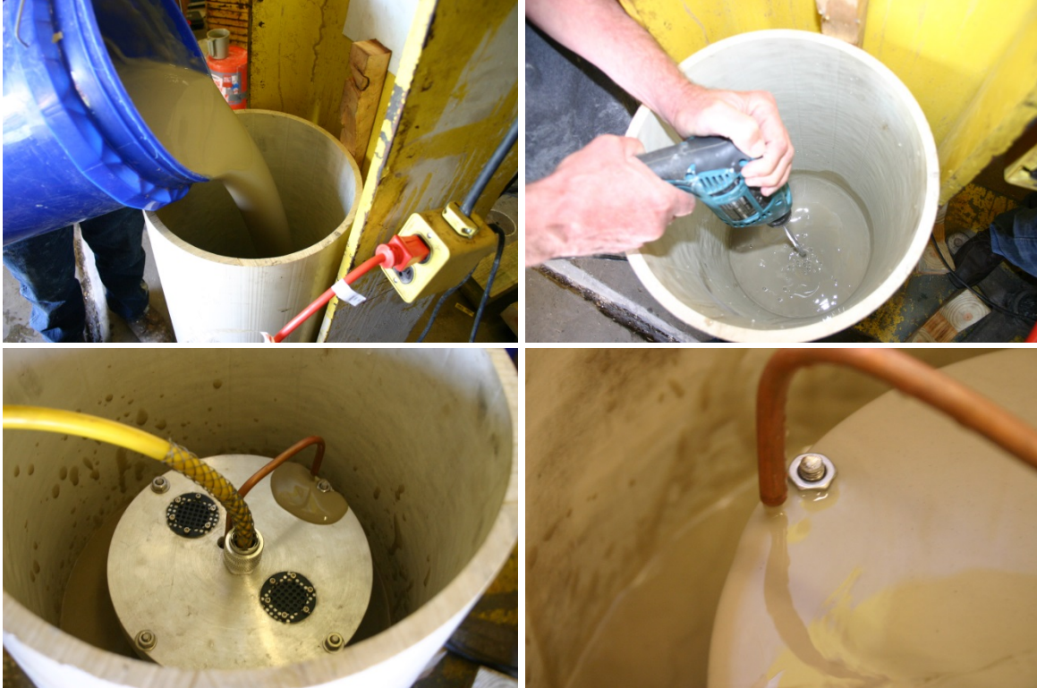
Figure 4.17. Slurry placed and stirred in calibration chamber (top); DHU partially submerged in bentonite during calibration (bottom).
