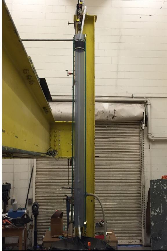
Figure 3.2. 115.25in tall falling head test column
