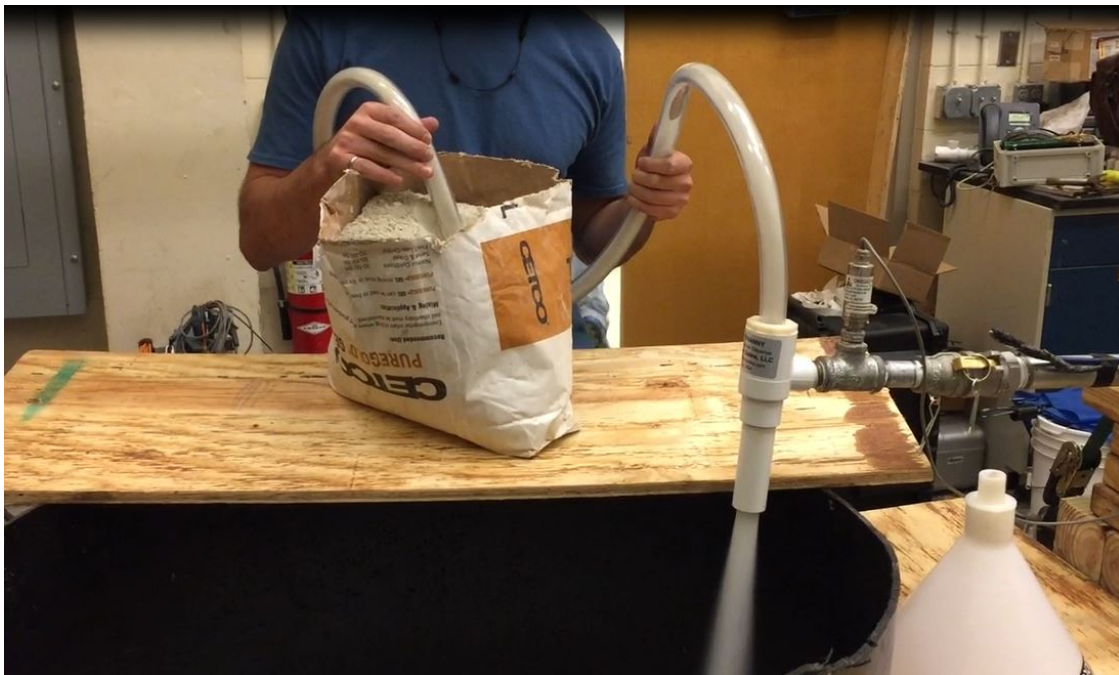
Figure 4.22. CETCO PURE GOLD GEL being mixed with Hootonanny eductor with vacuum tube feed.
