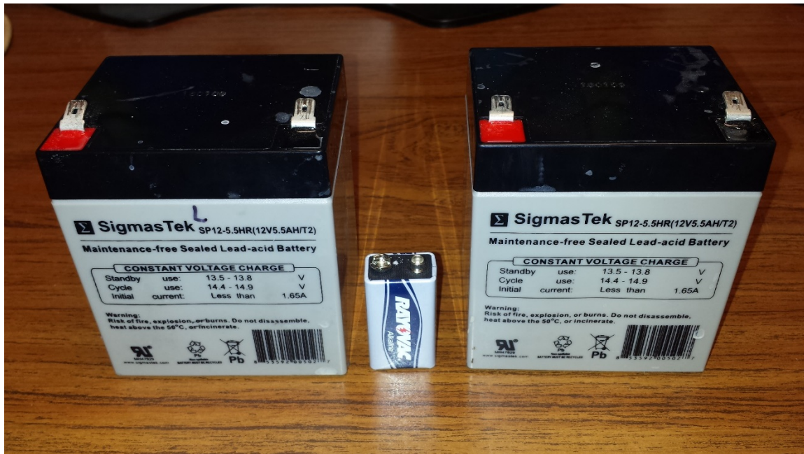
Figure 4.6. 12 volt batteries with common 9 volt for size reference.
