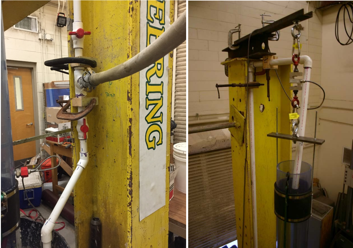
Figure 3.9. Slurry mixing/delivery system flow valves and slurry discharge point at top of tube
