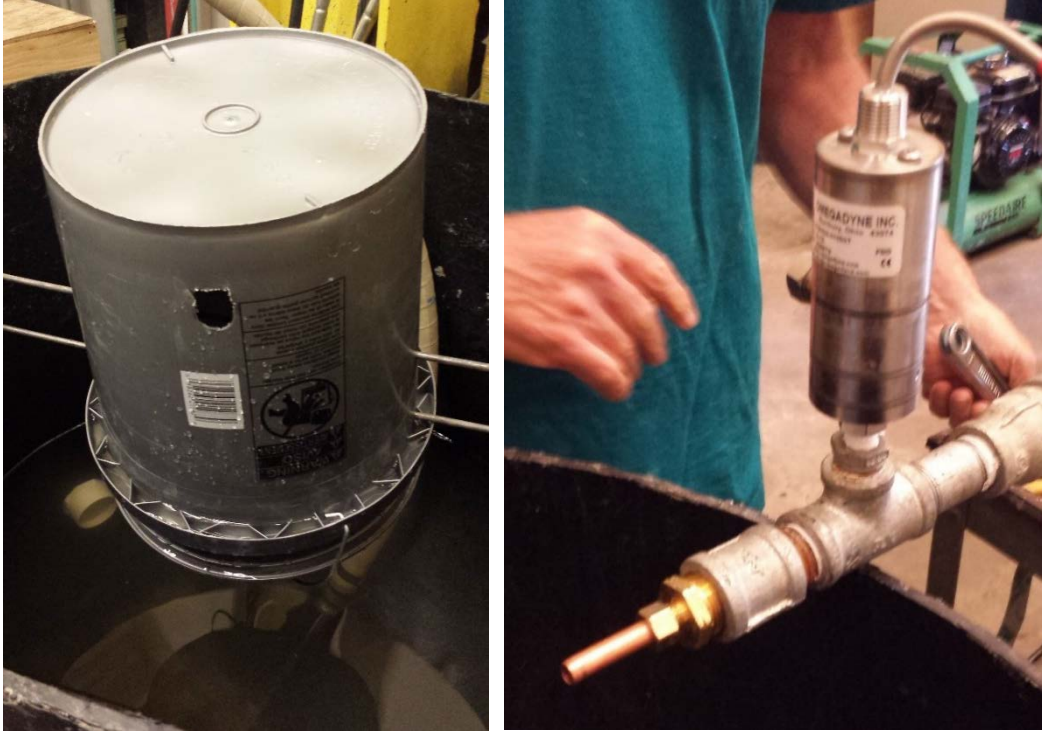
Figure 3.54. Bucket to return discharge flow back into tank and 0-10 psi pressure transducer
