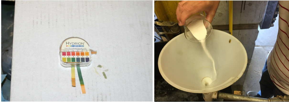
Figure 3.10. Mixing water pH test before and after introduction of soda ash through Hootonanny eductor
