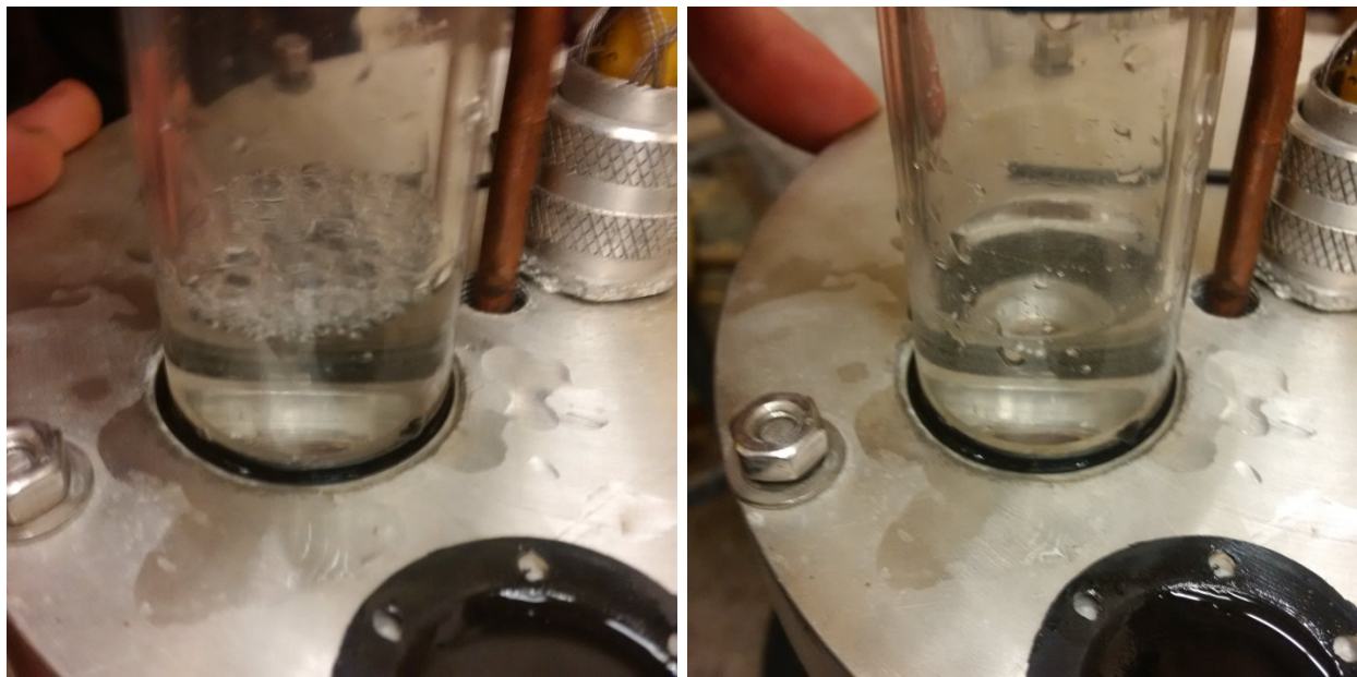
Figure 5.7. Vacuum purging of low pressure density pressure port with glycerin solution; initial (left), after 15min under vacuum (right).
