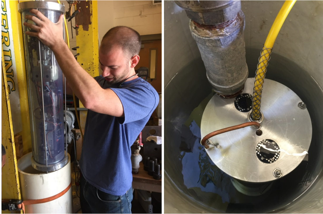
Figure 4.16. DHU submerged in clear water for buoyancy and first P vs F calibration test.
