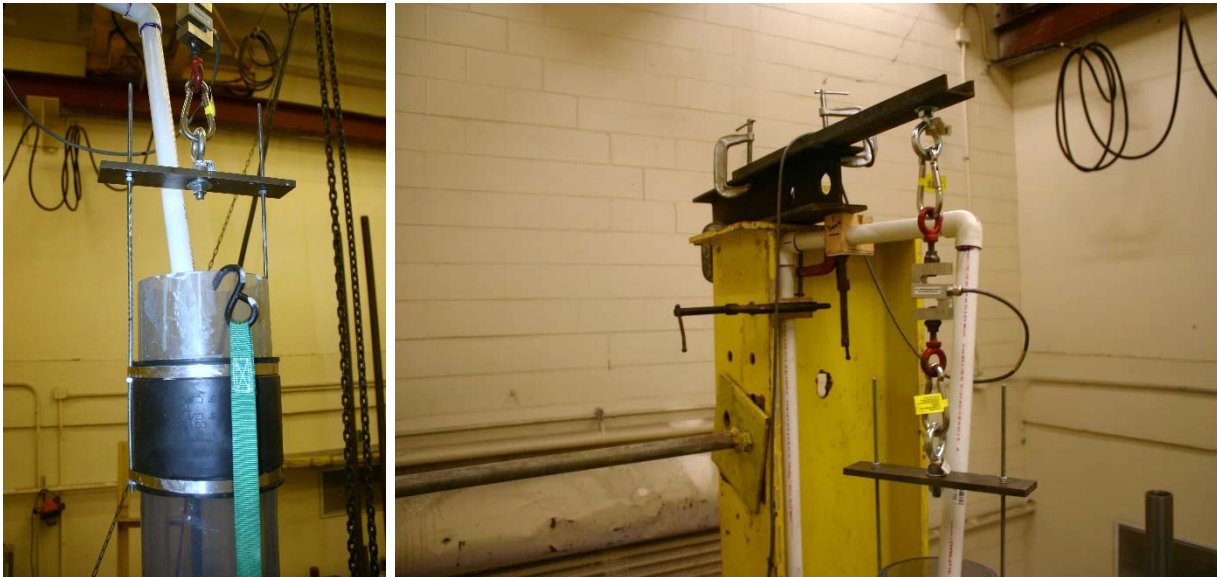
Figure 3.4. Falling head test tube system suspended from 15 foot tall column
