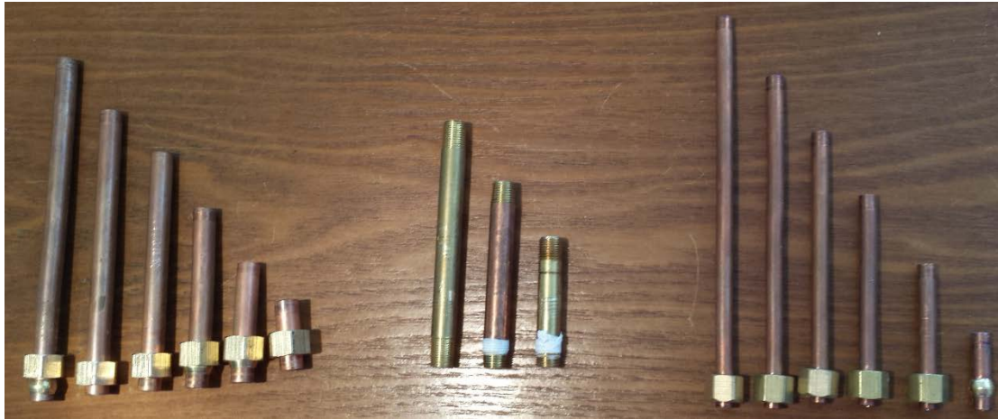
Figure 3.56. Varying lengths and diameters of orifices
