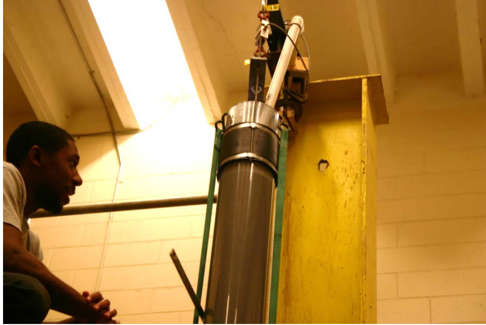
Figure 3.13. Filling test tube to level 9.5in from top of tube
