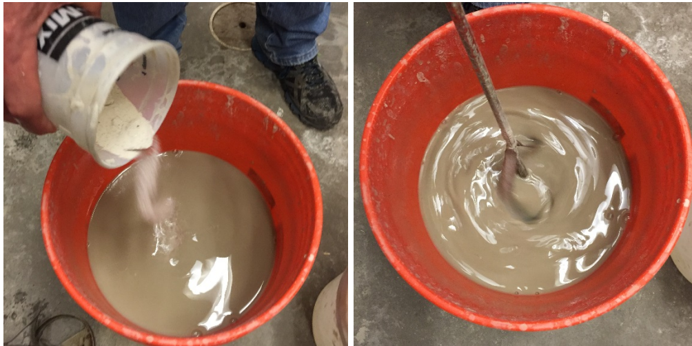
Figure 4.23. Adding sand to increase sand content to 2% then remixing slurry.
