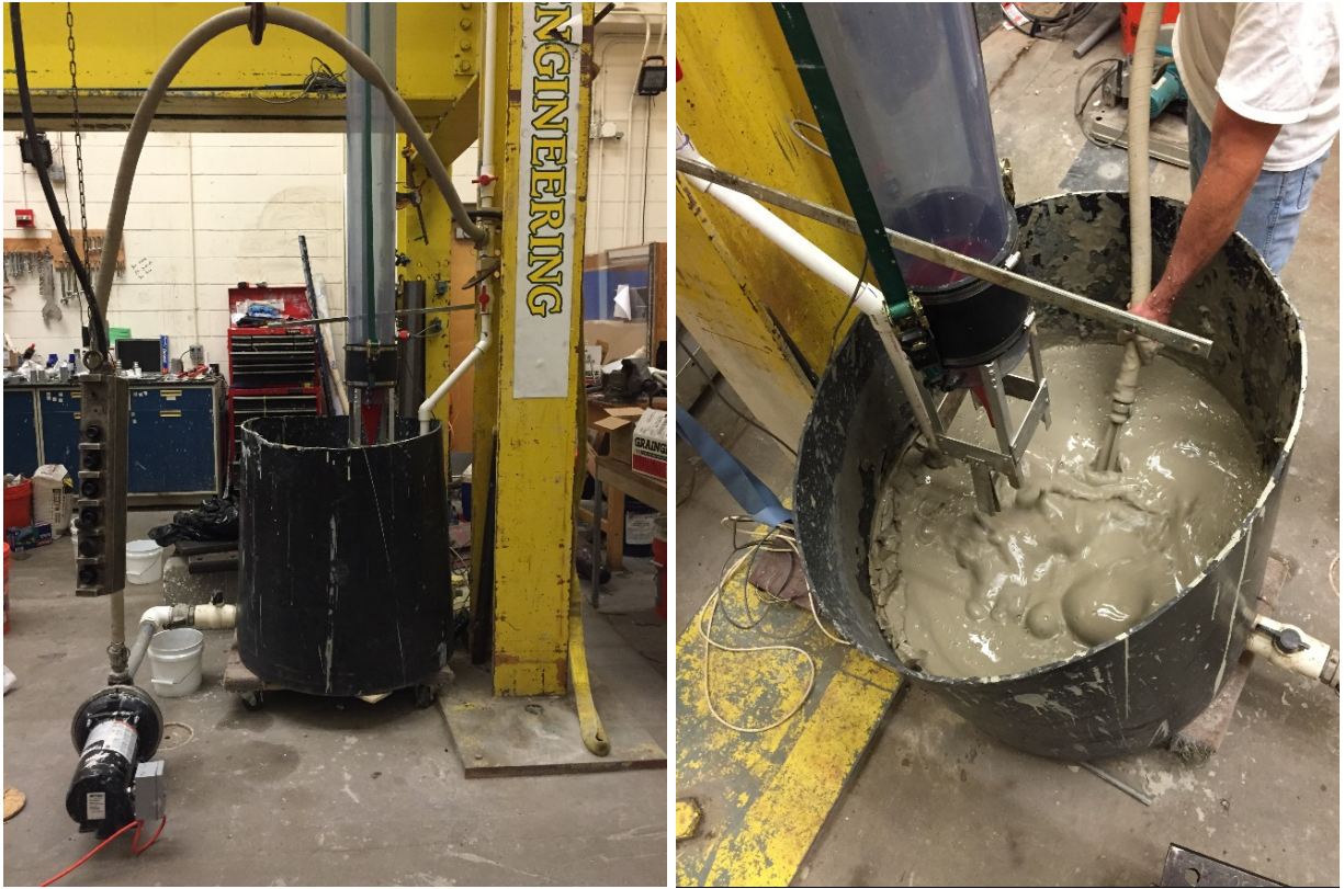
Figure 3.8. Slurry mixing/delivery system with system discharging to holding tank
